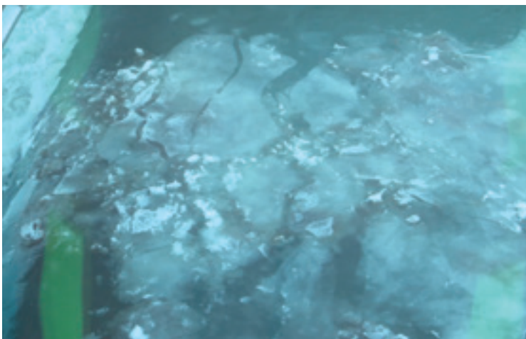
Released anchor ice rising to the surface. Photo courtesy New York Power Authority.
