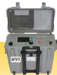
VLF 0.1 Hz @ 34 kVac Computer control - wireless
