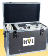
50 kVac @ 3 kVA Hipot 1 piece & w/cable output
